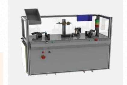
Operator intervention only in the beginning and operation ending / Checking piece version / Manual placing of the elements in the equipment / Checking sensors assembly through infrared view cameras / Checking OK by hot point regarding piece version / LED`s panel for error identification
