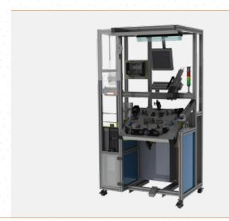
Check presence and position of several elements / Enables bolting with handle door torque control / Check the type of tissue used on the armrest by artificial vision / Bar code reader for the reference produced / Label print with final bar code
