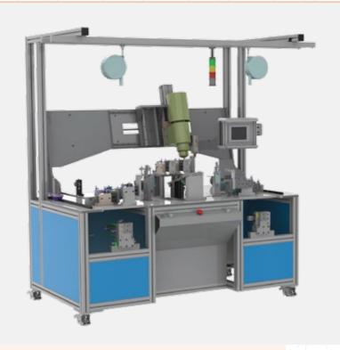
Equipment specially designed for placing metallic rivets on the plastic front end of the VW Passat Coupe.
