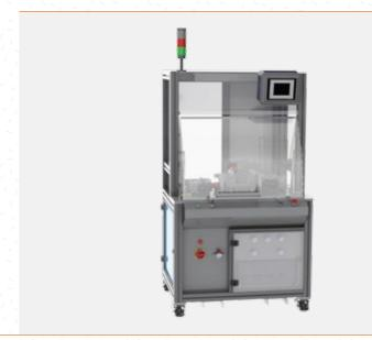
OK warning, when the piece is correctly welded / Frontal protection system / 5 sonotrodes / Console for process control and welding parameteres introduction
