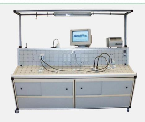
Equipment for high voltage test of small helicopter electrical wiring.
